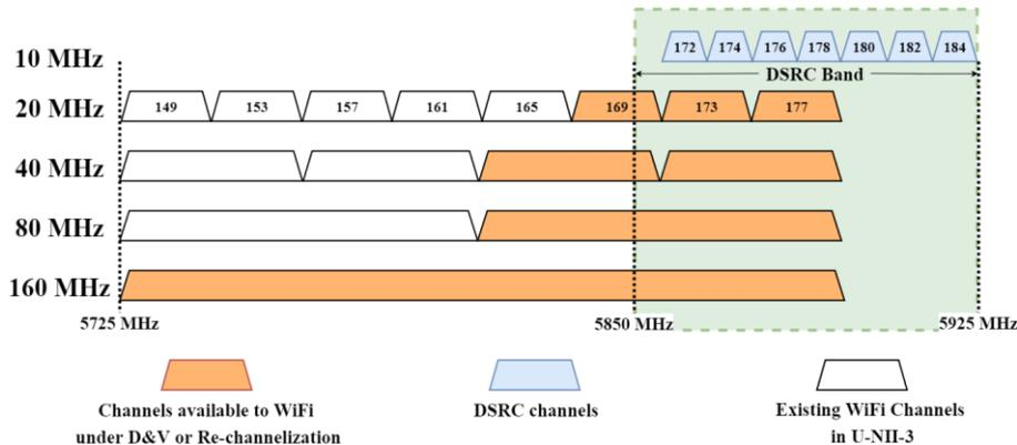
Figure 1 – An illustration of spectrum sharing in DSRC band
