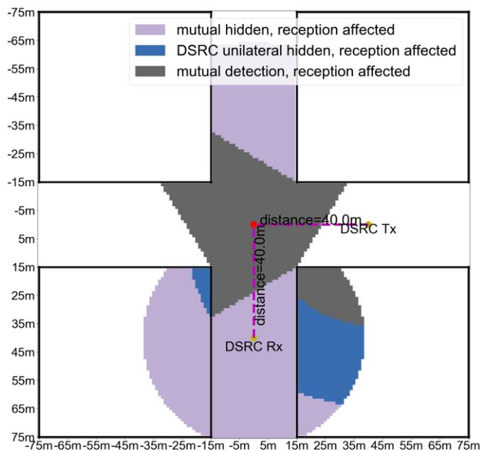
**Figure 6 - Potential impact regions on the DSRC performance with Wi-Fi device at various locations**
