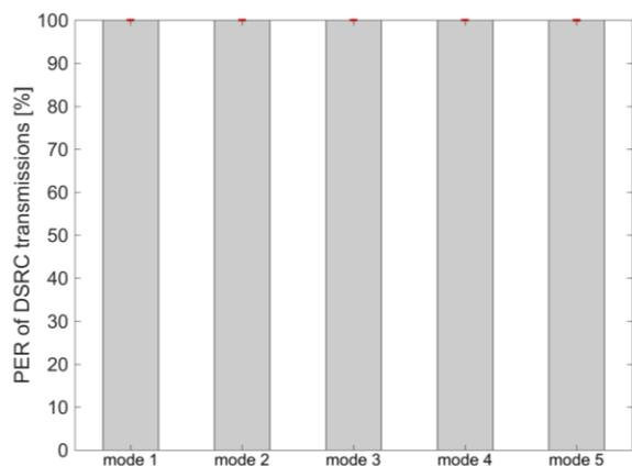
**Figure 4 – PER of vehicle 1’s transmissions due to hidden terminal problem**
