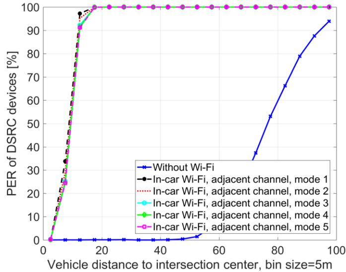
**Figure 3 - PER for vehicle 1’s BSMs sent to vehicle 2, with/without Wi-Fi present on adjacent channels**
