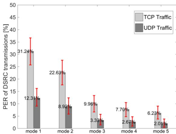
**Figure 7 - Packet loss of DSRC transmissions due to backoff countdown collisions between DSRC and Wi-Fi, TCP and UDP traffic**
