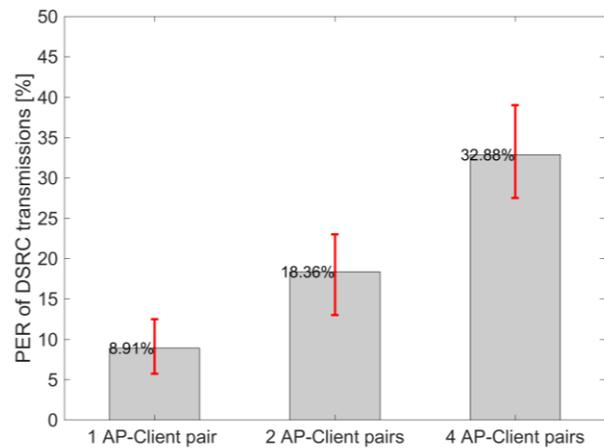
**Figure 8 - Packet loss of DSRC transmissions due to backoff countdown collisions between DSRC and Wi-Fi for the Re-channelization mode 2 with different numbers of AP-Client pairs, UDP traffic**
